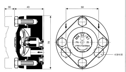
Thermostatic steam trap unit for low condensate flowrates, provided with corrosion-resistant thermostatic capsule unaffected by waterhammer. For mounting to an existing swivel connector. With integral strainer. Installation in any position.
